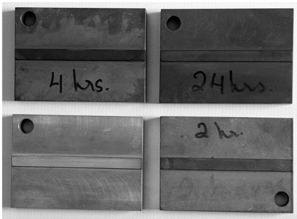
Figure 6. Surface Finish on Test Pieces after Heating to 480°C for Different Times Top Row : 4 hours, 24 hours Bottom row : Initial state, 2 hours
