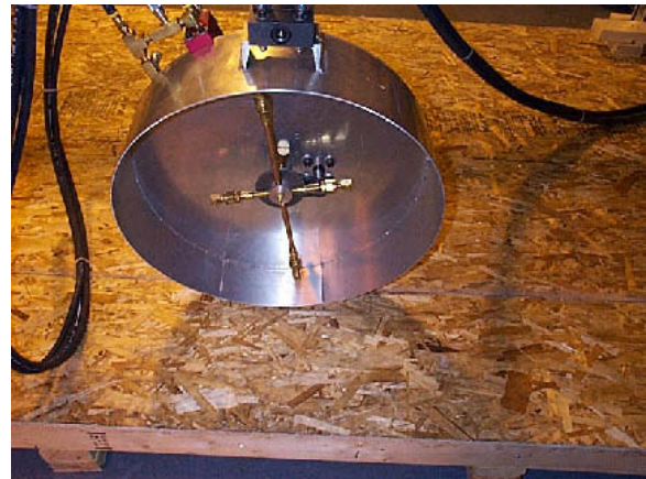
Figure 5: Rotating nozzles are driven with an air driven gear motor for improved system reliability.
