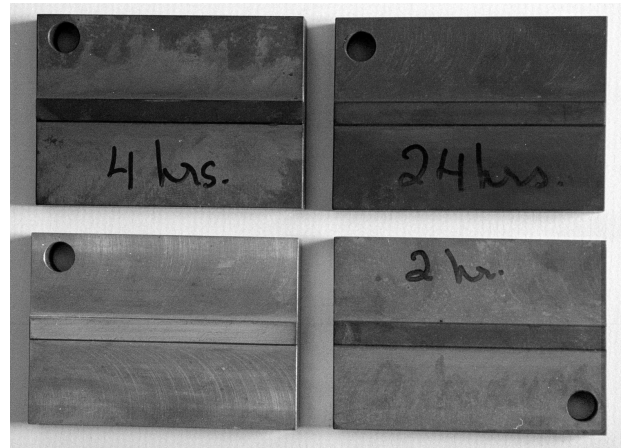
Figure 4. Surface Finish on Test Pieces after Heating to 480°C for Different Times Top Row : 4 hours, 24 hours Bottom row : Initial state, 2 hours
